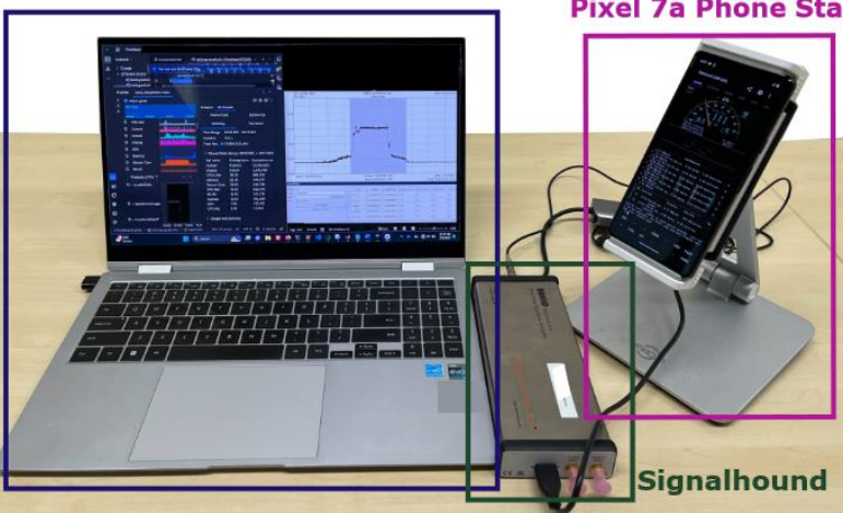
Laptop interfaces to Pixel phone via ADB and SignalHound via Spike software
