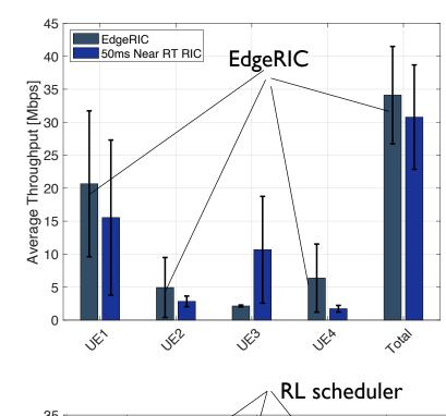
Providing scheduling control in real time indeed supports a higher system throughput
