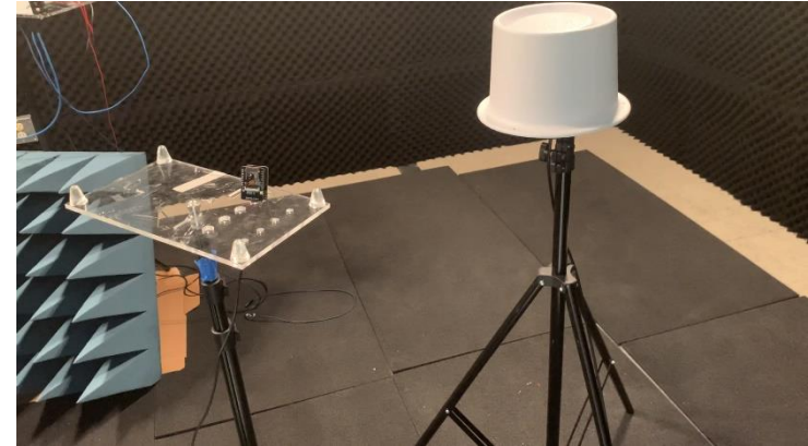
Anechoic RF environment for calibration and measurement
